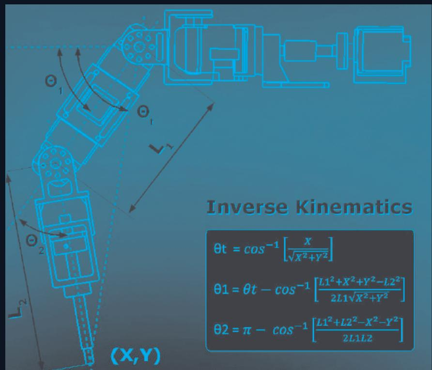
Figure 1: Robot spider leg appendages  $L_1$  and  $L_2$  tilt along angles  $\theta_1$  and  $\theta_2$ . Accelerometers in the appendages sense the tilt and feedback the position data to the inverse kinematics equation. Appendage  $L_1$  also rotates along  $\theta_1$ . (Source: Analog Devices)
