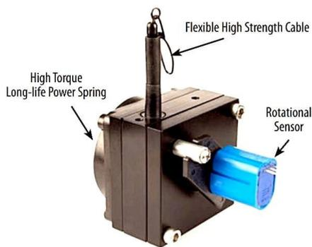
Figure 4: This draw-wire displacement sensor from Bourns shows the spring-loaded spool on which the cable is wound and a rotational sensor mounted to the enclosure. Several types of sensors can be used depending on the requirements of the application. (Source: Bourns)
