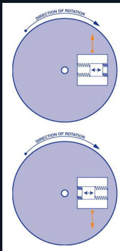
Figure 2: Internal operation of a MEMS gyroscope sensor (source: Analog Devices)
