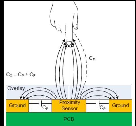
Figure 4 : A Cypress CapSense Proximity Sensor Coupling Electric Field Lines to a Finger. (Source: Cypress)
