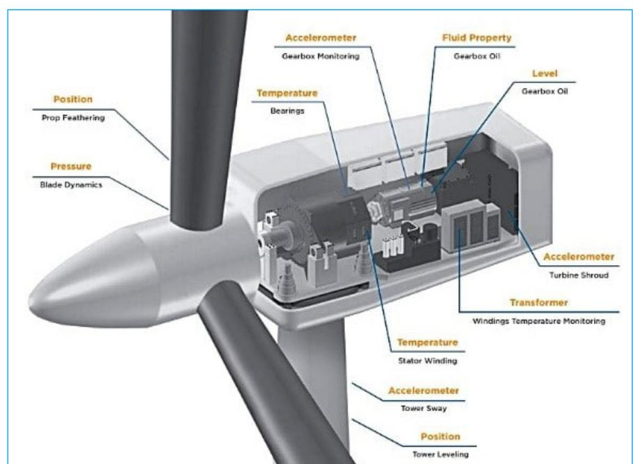
Figure 1: The basic components of a wind turbine within the nacelle and some of the types of sensors and where they're placed. (Source: TE Connectivity brochure)
